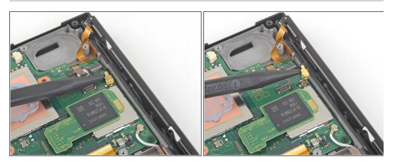
• Use the point of a spudger to pry up the black antenna cable straight up out of its socket on the motherboard.
