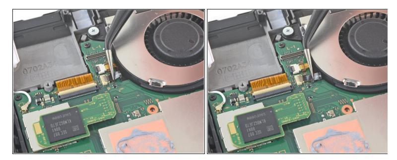
• Use a pair of tweezers to pull the fan cable straight out of its connector on the motherboard.
