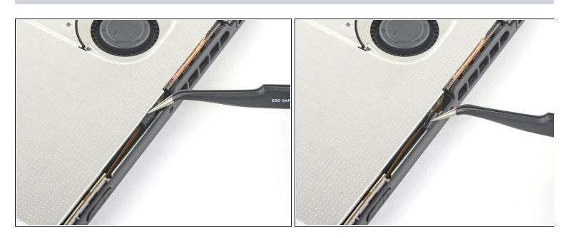
Use your fingers or a pair of tweezers to peel back the piece of foam on the top edge of the device near the fan exhaust port.
