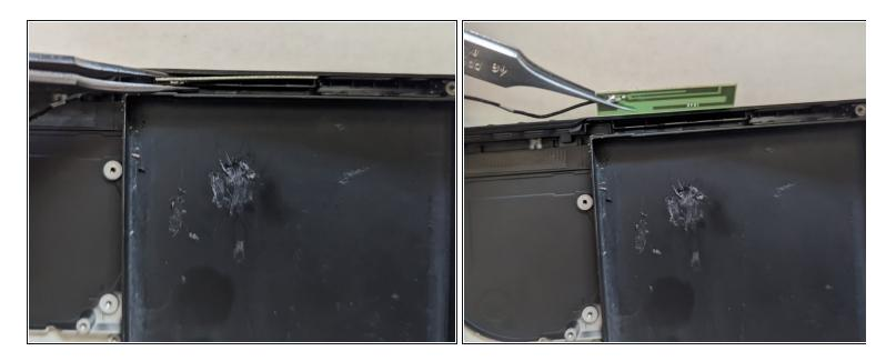
• Grasp the WiFi antenna board with a pair of tweezers and lift straight up to remove it.
