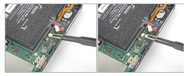
• Use your fingers or a pair of tweezers to pull the left speaker connector straight out of its socket on the motherboard.
