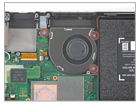
Use a JIS 000 screwdriver or an official iFixit PH 000 driver to remove the three 4.8 mm screws securing the fan.
