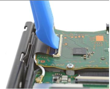
• Use an opening tool or your fingernail to flip up the small, hinged locking flap on the digitizer cable's <u>ZIF connector</u>.
