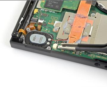
• Use your fingers or a pair of tweezers to pull the right speaker connector straight out of its socket on the motherboard.
