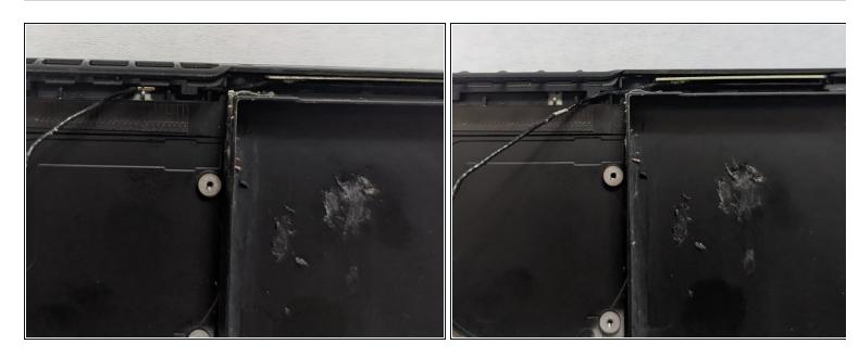
• Pry the metal barrel surrounding the coax up from the midframe.
