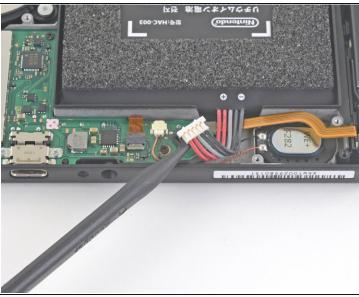
• Use the point of a spudger to pry the battery connector straight up and out of its socket on the motherboard.
