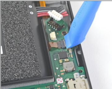
Use an opening tool, spudger, or your fingernail to flip up the small, hinged locking flap on the Joy Con sensor rail data cable <u>ZIF connector</u>.
