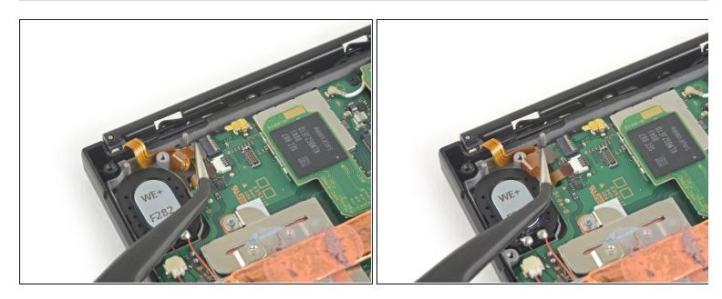
• Use a pair of tweezers to pull the ribbon cable straight out of its connector on the motherboard.
