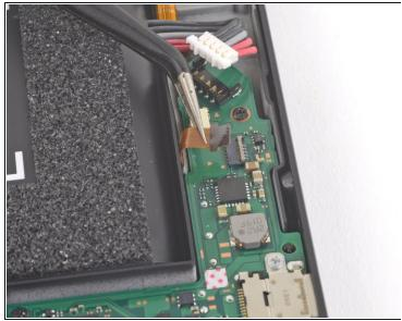
Use a pair of tweezers to slide the Joy Con rail data cable straight out of its connector on the motherboard.
