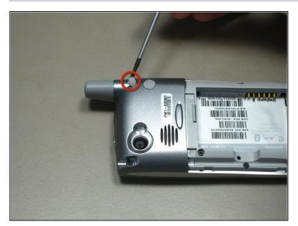
Remove the round, rubber cover to expose a screw that will be removed in the next step.
