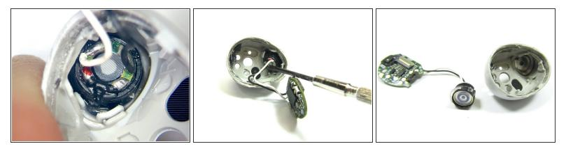
• Now we can remove the speaker from the headphone. The speaker is held in place with double side foam tape, so it best to use an Xacto knife to cut around the speaker. Then the speaker can be pried out with a small flathead screw driver
