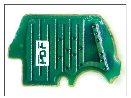
Pulling off the double sided foam tape, we can see the Touch Sensor and Bluetooth Antenna structure
