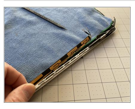
Lift up the antenna board up and out of the display.
