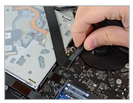
Use the flat end of a spudger to carefully pry the AirPort/Bluetooth ribbon cable up off its socket on the logic board.
