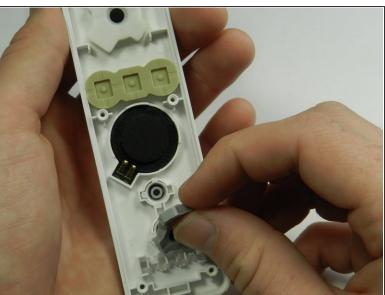
Working on the inside of the front cover, peel off the three rubber pads covering the buttons.
