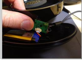
Contains a battery and connector PCB. Battery type is 603040 lithium ion, dimensions are 6mm thick X 30mm tall X 42mm wide, with a 3-pin JST (includes thermistor apparently)
