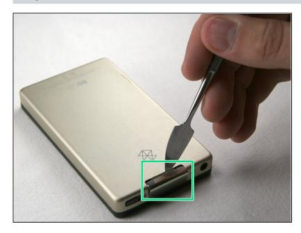
Use a metal spudger or Zune opening tool to remove the small silver plastic cap on top of the device.
