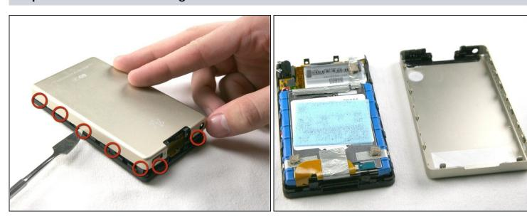
• Using a metal spudger or Zune opening tool, remove the aluminum backing starting from the top. There are 5 clips on each side and two on the bottom.
