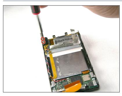
Remove the two T4 screws holding the headphone jack receiver on the top left corner of the device.
