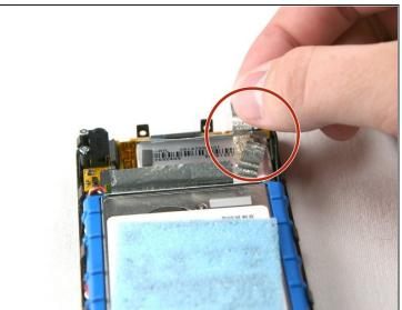
• Remove the silver tape from the bottom center and the top right. This allows access to the hard drive and the battery.
