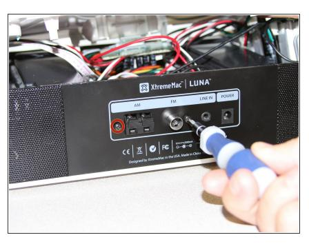
Remove the two 12mm Phillips head screws from the back of the device using a Phillips #1 screwdriver.
