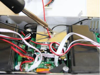
Desolder the positive connection (red) and the negative connection (black) on top of the radio jack to completely remove it.
