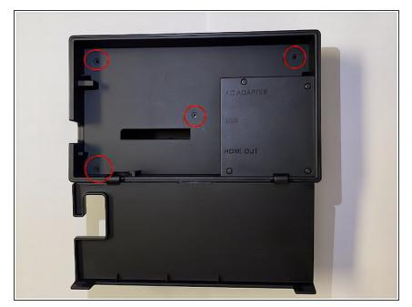
Use Tri-head driver to reinsert screws (1, 2, 3, 4)
