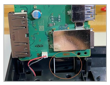
Gently pull the film cable out of the circuit board. The cable should slide free when lightly pulled.
