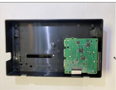
Carefully pull to remove the backing from the switch dock, exposing the circuit board.
