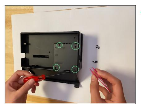
Use Tri-Head driver to reinsert screws (A, B, C, D)
