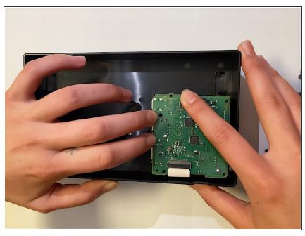
Gently apply pressure to the circuit board to ensure it seats into the housing.
