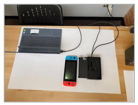
Plug HDMI cable into a device with an HDMI port (TV, monitor, computer, etc.) (NOTE: need adapter for PC for video and audio connection)
