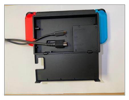
Unclip the back plate. It will fold back to expose the power wire and the HDMI cable.
