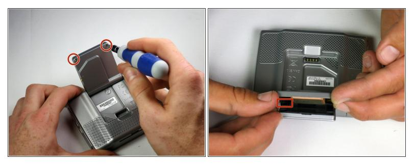
Unscrew the two screws on the antenna unit using a torc-head screwdriver.
