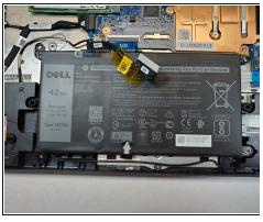
Use a spudger to disconnect the battery cable from the motherboard located at the top of the battery.
