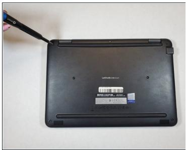
• Use a Phillips #0 screwdriver to remove the seven 7 mm screws securing the back case.
