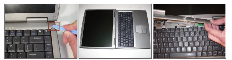
Use a spudger to lift the notched right edge of the hinge cover, and pry it loose
