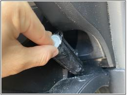
Unhook the damper arm connected to the glove box.
