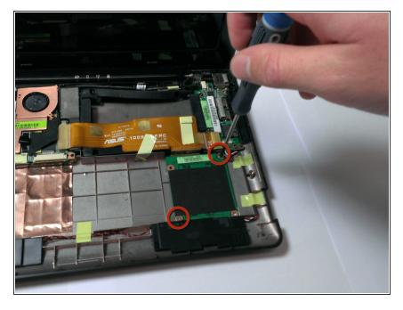
Remove the two 2mm screws from the graphics card.
