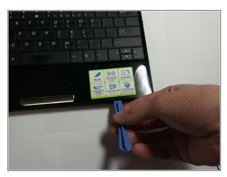
Using the plastic opening tool, carefully pry the top panel from the base.
