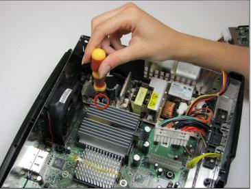
Using T10 Torx screwdriver, remove two 3mm screws from the tan power supply board.
