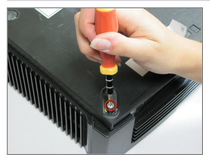
Remove the six T20 Torx screws securing the top cover to the bottom cover.
