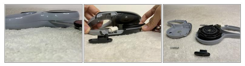
• Using a plastic opening tool, begin to separate the top and bottom of the leash.
