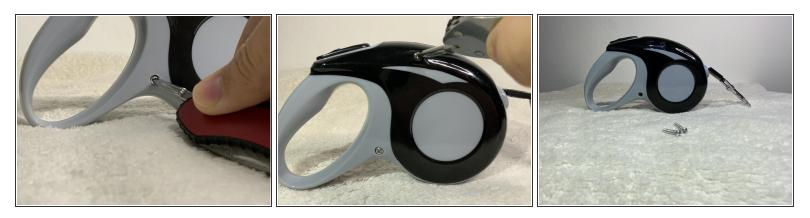
• Start by removing all the 0.5 cm screws off the leash with the Phillips #0 screwdriver.
