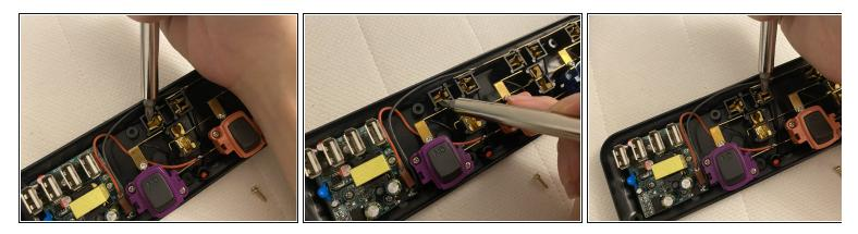
• Use a screwdriver to push the two copper sheets closer to each other. Do this on all the pairs of copper sheets without a solid connection.
