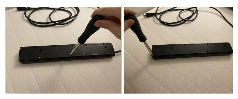
• Flip over the power strip, and then use screwdriver to install all the screws back.
