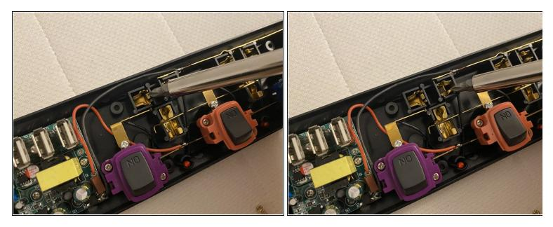
• Locate two pairs of copper sheets for each socket.
