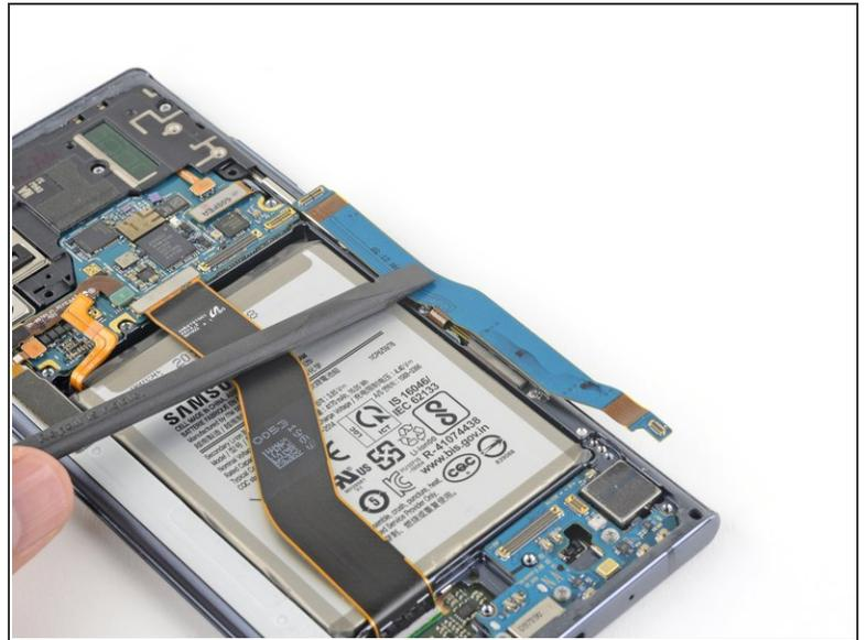
**⚠ Don't try to remove the secondary interconnect cable. The cable is connected to the side 5G mmWave antenna.**
