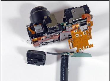
• Lift the entire three-part flash assembly from the camera.
