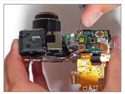
With a Phillips #00 Screwdriver, unscrew the flash board.
