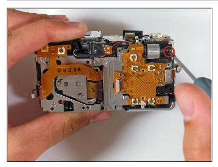
With a Phillips #00 Screwdriver, unscrew the zoom toggle switch and remove it from the camera.
