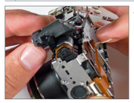
Lift the flash bulb unit upwards from the camera.
