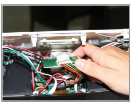
Unscrew the four black 7mm screws with the Phillips #1 screw driver that hold the middle circuit board to the top case.
