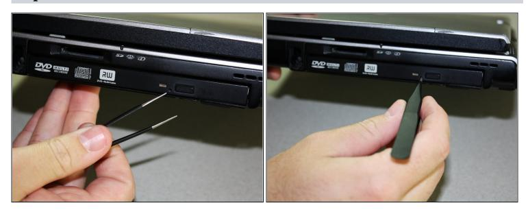
• Using the <u>tweezers</u>, insert them into the small hole next to the CD drive button.
