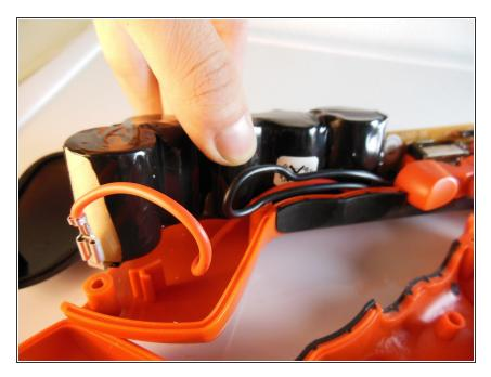
Locate the battery and remove it from its slot at the end of the drill opposite the motor. It should be at the butt of the drill by the handle.
