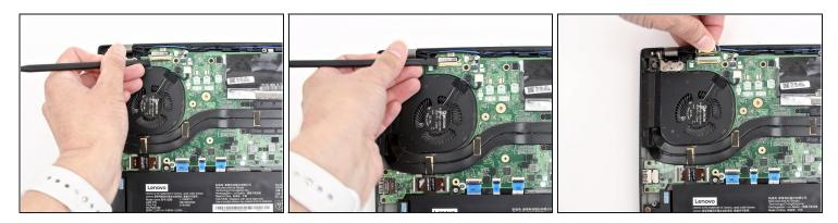
• Disconnect the camera cable from the motherboard using a spudger.
