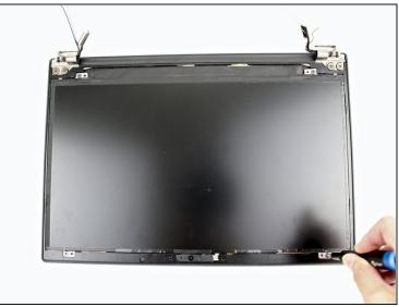
• Remove four 2.9 mm screws from the LCD panel using the Phillips #1 screwdriver.
