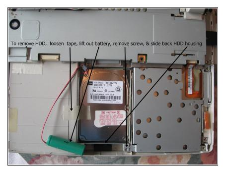
To remove HDD loosen tape, lift out BIOS battery, remove screws and slide back HDD housing.
