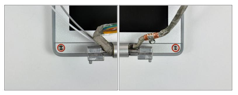
Remove the two 5 mm Phillips screws from the lower left and right corners of the display (two screws total).
