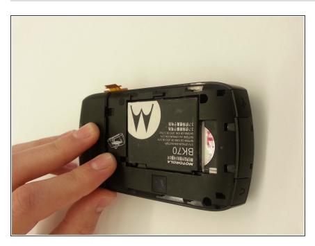
Remove the battery cover of this device by sliding it down and then lifting it up.
