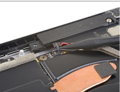
• Use the point of a spudger to lift the right speaker connector out of its socket on the motherboard.
