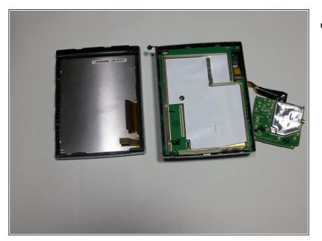
After following the instructions in the main dis-assembly guide, you should have the screen detached from the motherboard.
