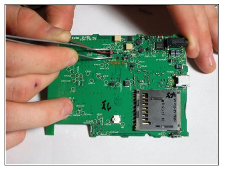
• Gently pull out the microphone wire from the terminal. Tweezers are recommended for precision.
