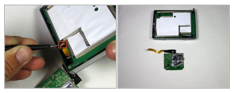
Use the tweezers or the spudger to lift the tan latch off the ribbon cable (ZIF connector) and gently pull out the ZIF connector and cable from underneath the opened latch.
