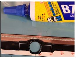
With the home button and bracket removed, apply liquid adhesive around the new glass digitizer's home buttonhole.
