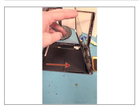
Lift the LCD screen from the top carefully.
