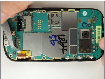
• Use <u>tweezers</u> to carefully remove the yellow piece of tape covering the two ribbon cables.
