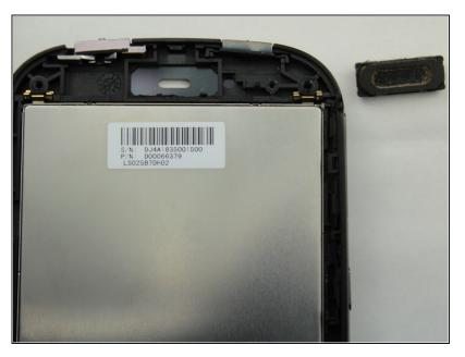
The speaker can be gently lifted off the phone and set aside for cleaning, repair, or replacement.
