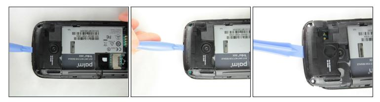
• Use a plastic opening tool to remove the small panel on the top of the phone by prying underneath the black plastic around the camera.
