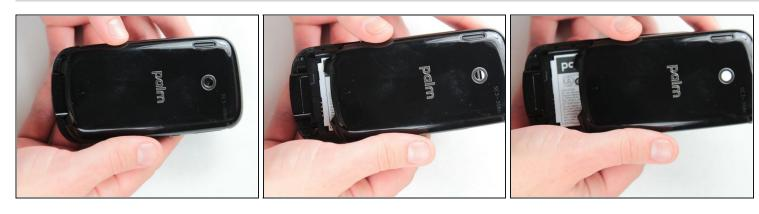
Press down on the back of the case and slide forward to remove it.
