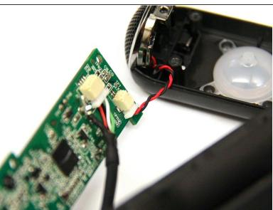
• Remove the four 6mm Phillips #0 screws connecting the motherboard and front cover.
