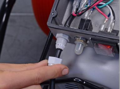
Slide the cap off of the strain relief fitting.
