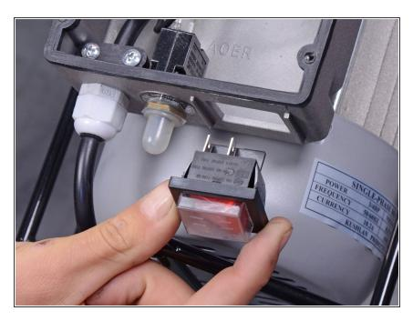
Remove the on/off switch.
