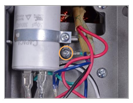
Use a Phillips screwdriver to remove the screw securing the green ground wire to the bottom of the electrical box.
