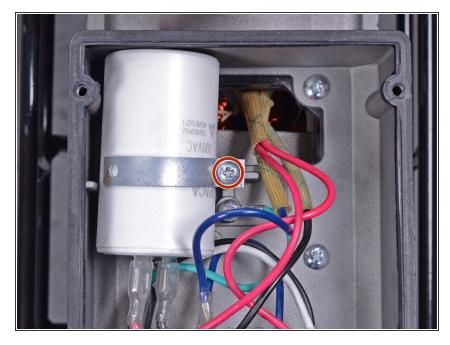
Use a Phillips screwdriver to remove the screw securing the capacitor support.
