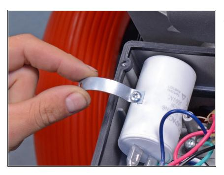
Remove the capacitor support.
