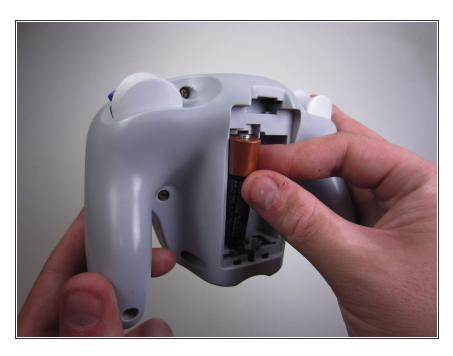
Remove both batteries from the device.
