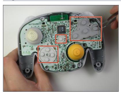
Using <u>tweezers</u> remove the three grey button pads from the motherboard.
