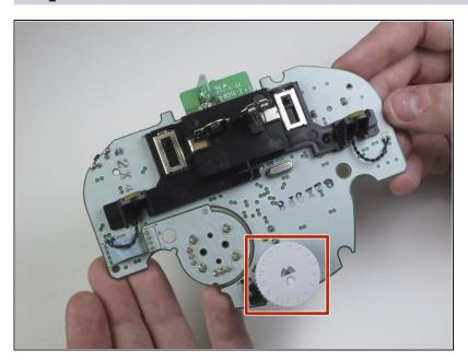
Turn the motherboard over so the channel wheel is facing up.
