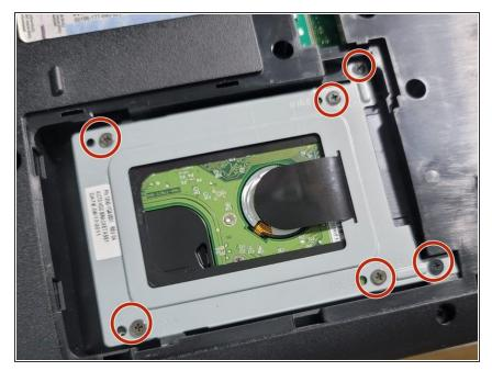
Using the Phillips #1 screwdriver, remove the six 1.2 mm screws holding down the hard drive.
