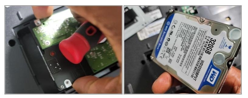
Remove the hard drive from the device.
