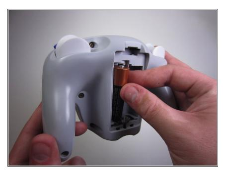
Remove both batteries from the device.
