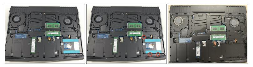
Remove the two M3x3 screws that are holding the bracket and one M2.5x8 screw holding the hard drive assembly.
