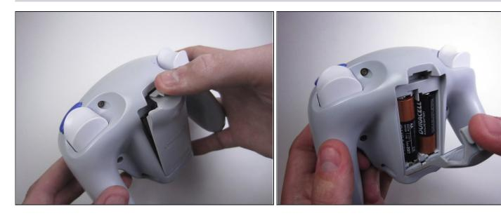
Pull down on the battery cover release lever and pull back to remove the cover.
