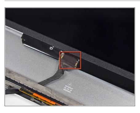
Peel the piece of tape covering the display data cable connector away from the edge closest to the LCD.
