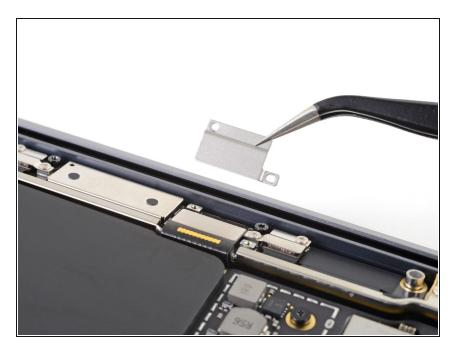
Remove the display cable connector cover.
