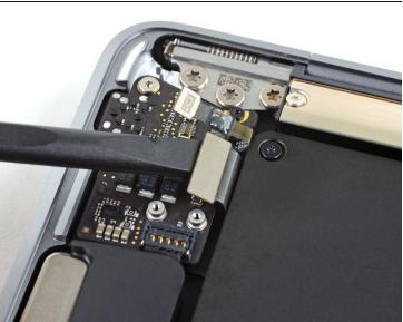
• Use the flat end of a spudger to pry the audio board connector straight up to disconnect it from the board.
