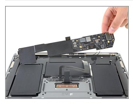
Remove the logic board.
