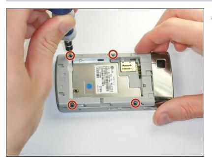
Using the #00 Philips screw driver, unscrew the four 4.5mm screws located around the battery compartment.
