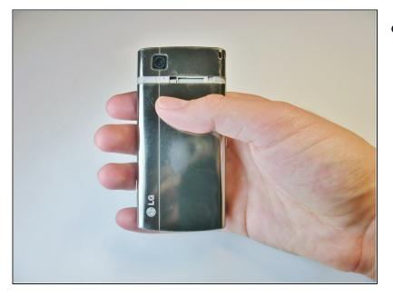
Place a thumb below the camera, apply a little pressure, and slide the cover toward the bottom of the phone.
