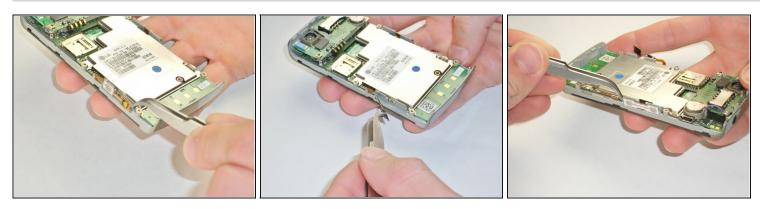
• Use the metal <u>tweezers</u> to gently peel the yellow tab from the left edge of the phone at the two plastic bases.
