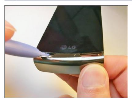
• Wedge the plastic opening tool under the screen where the buttons were to loosen it.
