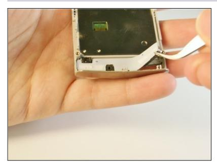
Remove the call and end buttons using the metal <u>tweezers</u>.
