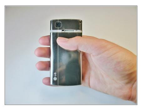
Place a thumb below the camera, apply a little pressure, and slide the cover toward the bottom of the phone.
