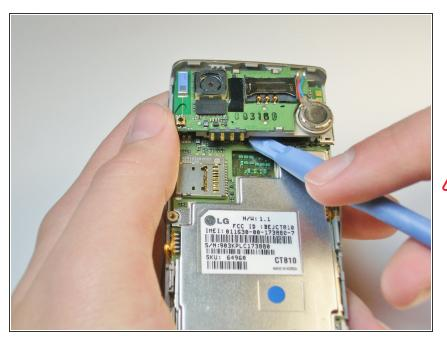
Insert your plastic opening tool underneath the speaker/camera panel, and gently pry it upwards.
