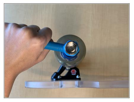
• Using a 15 mm socket wrench, unscrew the axle nut.
