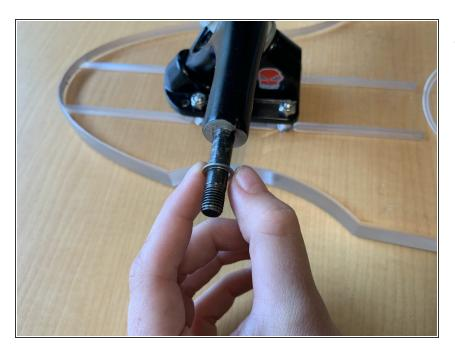
• Slide a new washer onto the axle.
