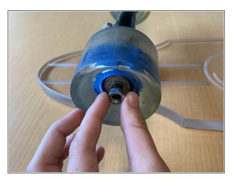
• Using your fingers, remove the axle nut from the axle.
