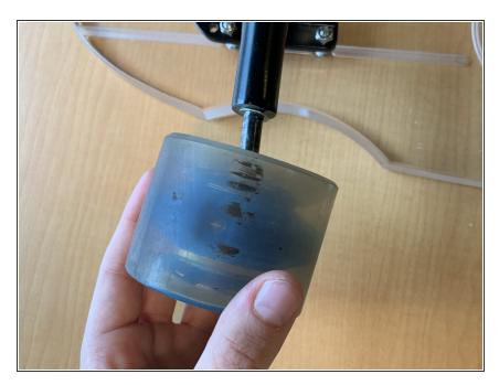
• Remove the wheel from the axle.
