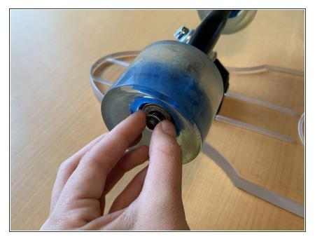
• Remove the washer from the axle.
