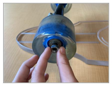
• Place an axle nut on the axle.
