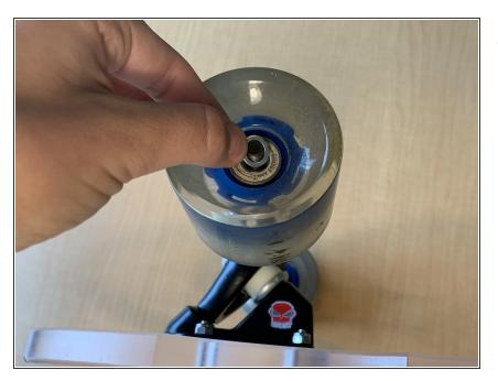
• Place a second washer on the axle exterior to the wheel.
