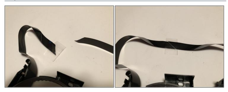
Apply scotch tape to the dull side of the two matching halves of the VHS tape.
