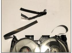
Cut out the wrinkled and damaged parts of the VHS tape using scissors.
