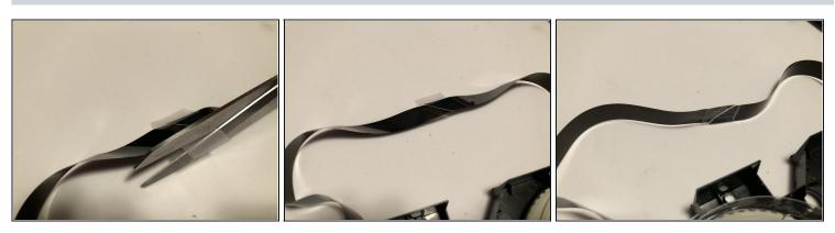
Cut excess scotch tape to match the size of the VHS tape as precisely as possible.
