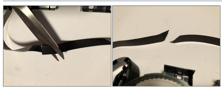
• Cut the overlapping portion of the tape at an angle.
