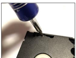
Remove the screws at the bottom of the VHS case using a Phillips #0 screwdriver.
