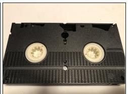
Reinsert the screws through the bottom of the VHS tape.
