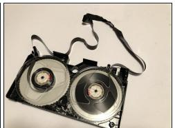
• Unroll the video tape from each side of the VHS, running it through the rollers the correct way. Do this until you reach the damaged parts of the tape.
