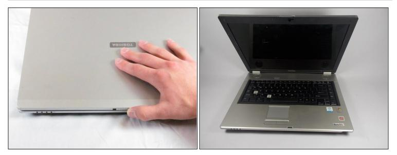
• Open laptop by sliding the front tab to the right and lifting the screen.
