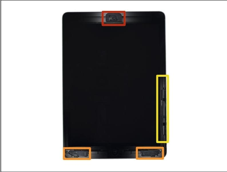
ⓘ While the iPad looks uniform from the outside, there are delicate components, such as flex cables, under the front glass. To avoid damage, only heat and pry in the areas described in each step.
