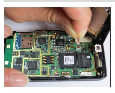
Gently pull the wire up from the motherboard, separating the back of the phone and the motherboard.
