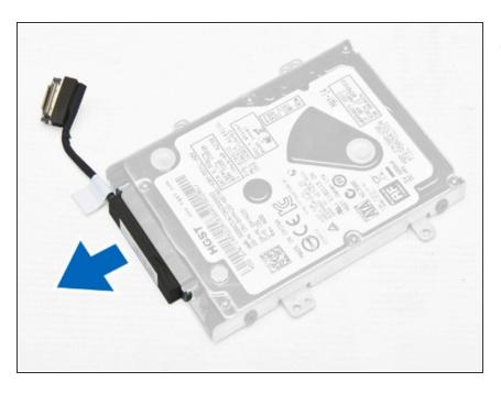
Pull to release the hard-drive cable from its connector.
