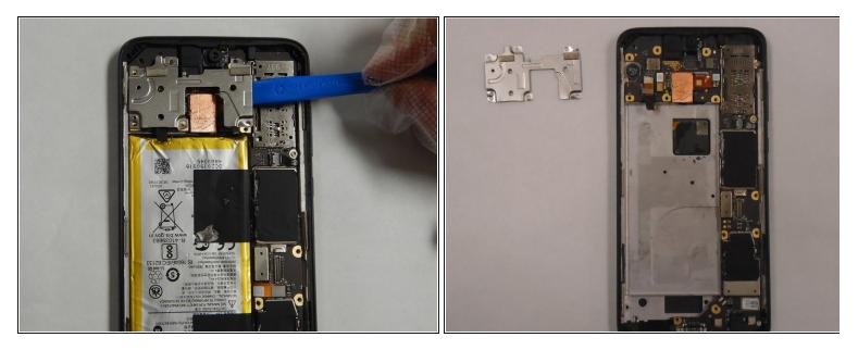
• Remove the camera housing plate with the opening tool.
