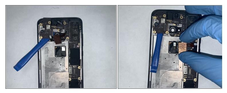
• Pry the motherboard away from the frame of the phone using the opening tools.
