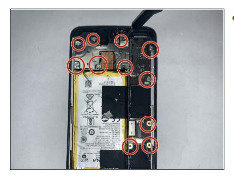
Remove the eleven screws with the T5 Torx screwdriver.
