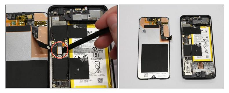
• Underneath this metal piece is the base of the cable. Use a spudger to vertically lift the connection out of its port.
