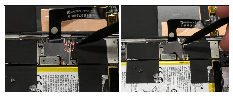
Use the pointed end of the spudger to lift the metal casing where circled.
