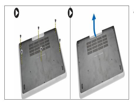
Remove the sides on the back of the computer to take off the cover for the battery.
