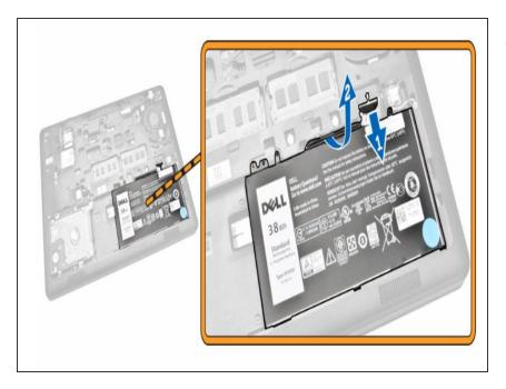
Disconnect battery cable from the connector and release cable from its routing channel.
