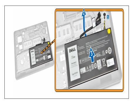
Remove the screw that secures the battery and lift and push to remove the battery from the computer.
